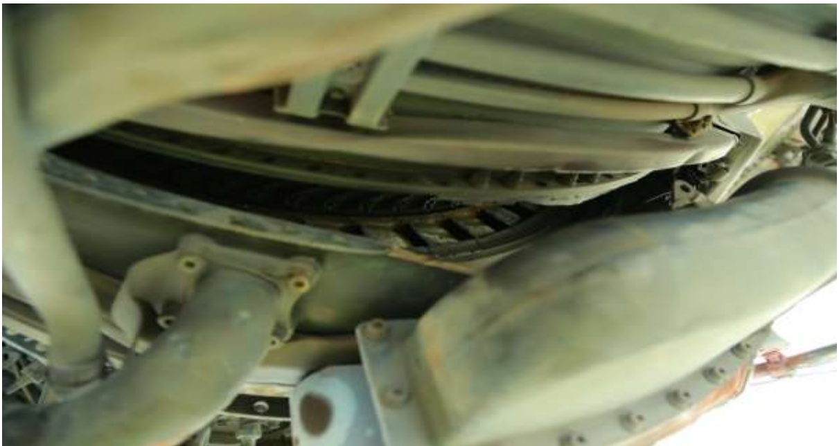
The High Pressure Turbine case breached
